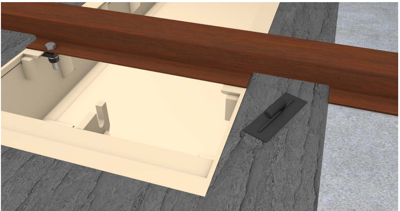
Trowel the concrete to provide a smooth, level approach on and off the weighbridge.
