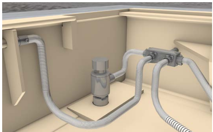
Connect the flex conduits from the frame and the load cells to the access port hub.
