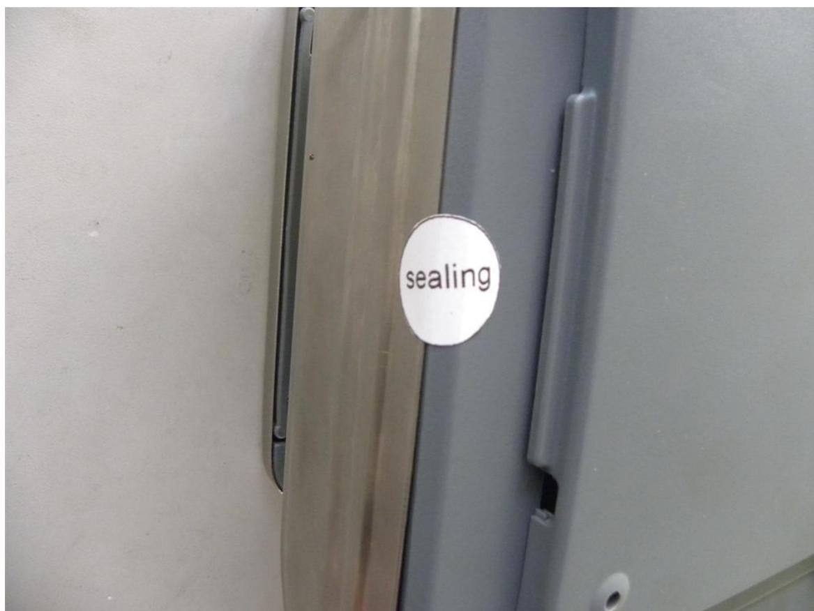
**Figure 3** Sealing of scale enclosure with brittle sticker.
