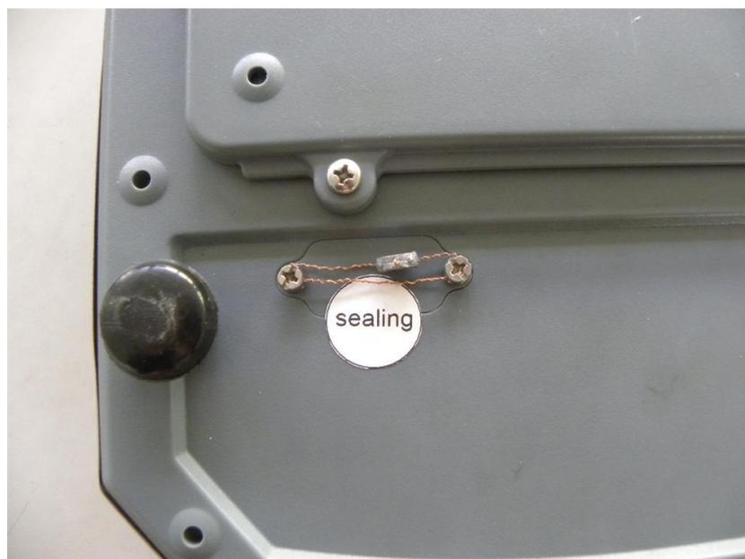
**Figure 2** Sealing of scale enclosure with wire and plastic seal in the rod and brittle sticker.
