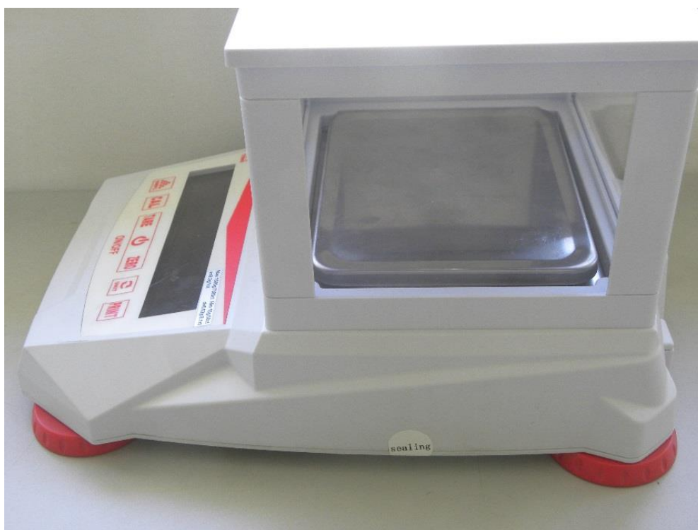
Figure 3 Sealing of scale enclosure with brittle sticker.
