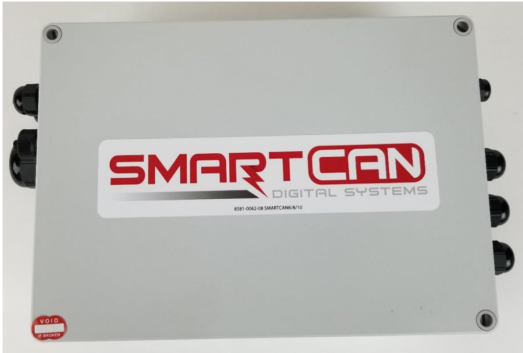
Figure 7 Sealing of enclosure for 10 LC system with tamperproof label
