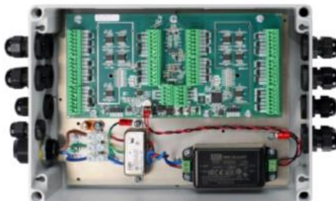
Figure 2 SmartCAN intended for up to 10 load cells with the optional power supply
