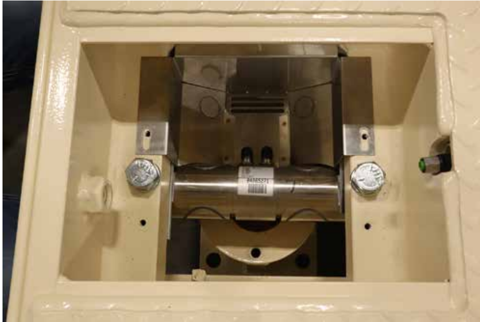
Figure No. 3 – First load cell guard installed and positioned over threaded holes.
