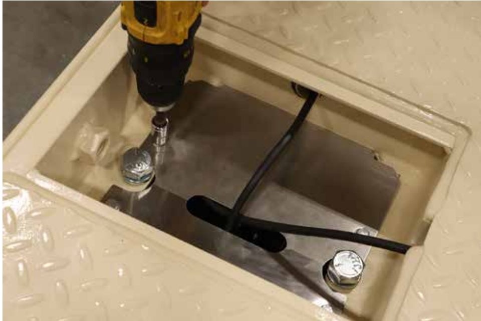
Figure No. 11 – Install four 1/4-20 x 3/4 in. hex head bolts to secure load cell guards and covers.
