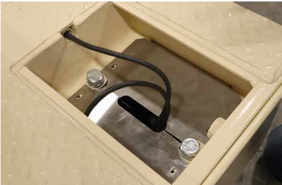
Figure No. 10 – Second load cell guard cover installed and positioned over threaded holes.
