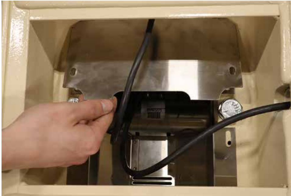
Figure No. 7 – Tilt the load cell guard cover at an angle and slide it under the load cell cable.
