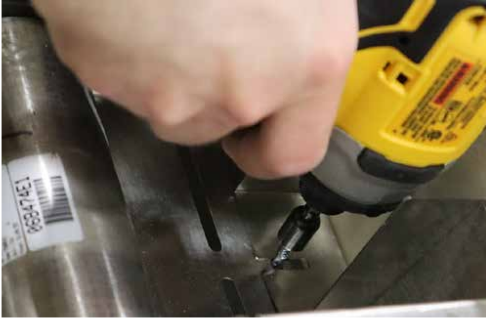
Figure No. 7 – Use the #10 x .75 in self-tapping screw to secure the inner guard plate to the inner load cell guard.
