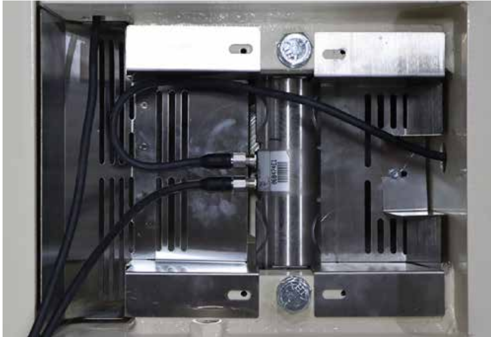
Figure No. 9 – Connect the digital load cell cables to the load cell.
