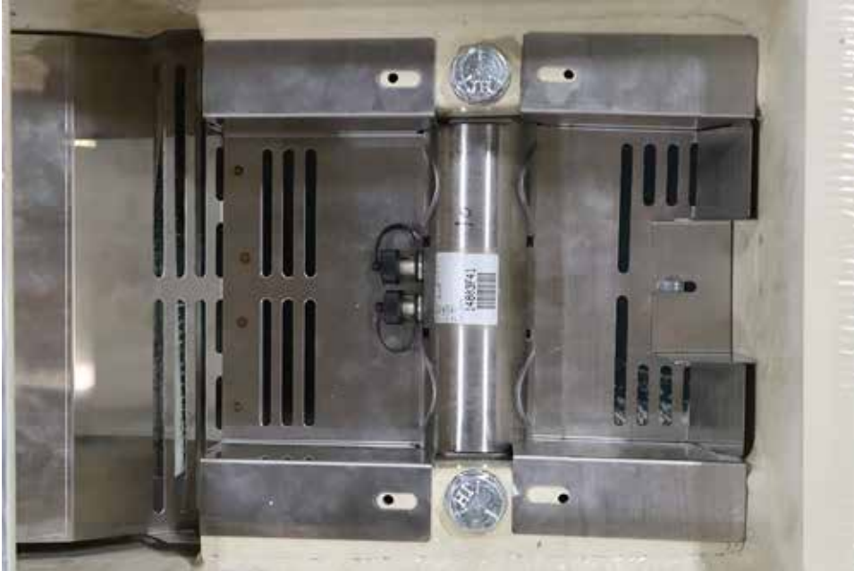
Figure No. 9 – Outer load cell guard installed and positioned over threaded holes.
