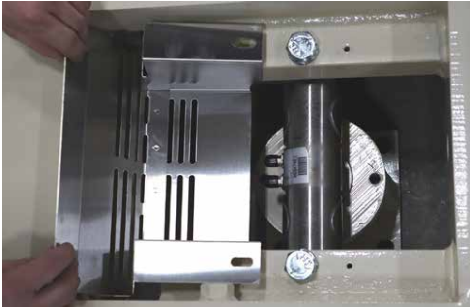
Figure No. 2 – Tilt outer load cell guard at an angle and slide under load cell cable connectors.
