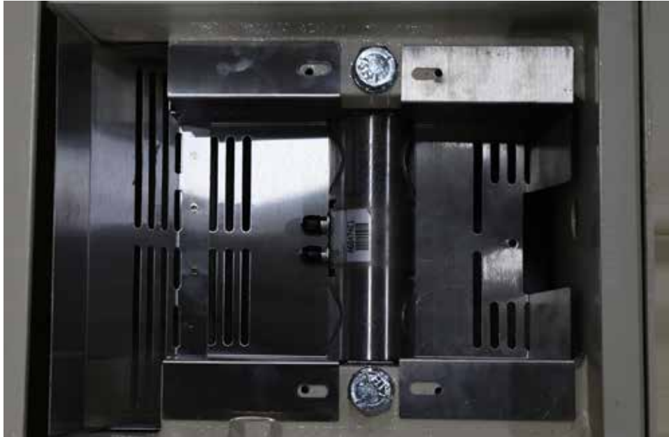
Figure No. 5 – Inner load cell guard installed and positioned over threaded holes.
