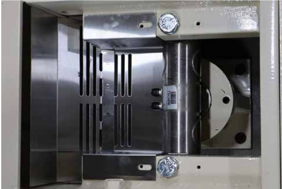
Figure No. 3 – Outer load cell guard installed and positioned over threaded holes.
