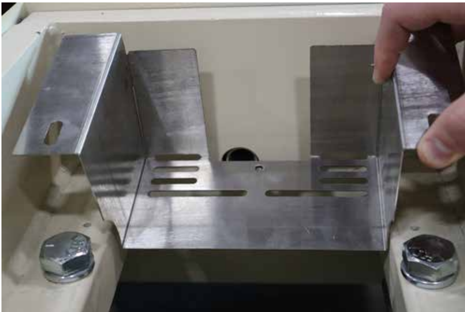
Figure No. 2 – Tilt the inner load cell guard at an angle, then lower it into the load cell pocket.
