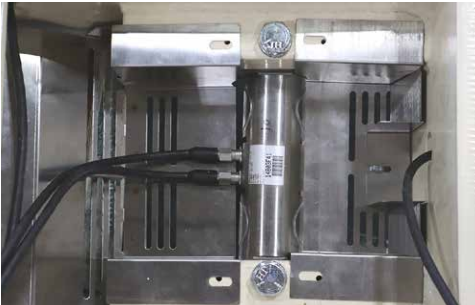
Figure No. 10 – Connect the digital load cell cables to the load cell.
