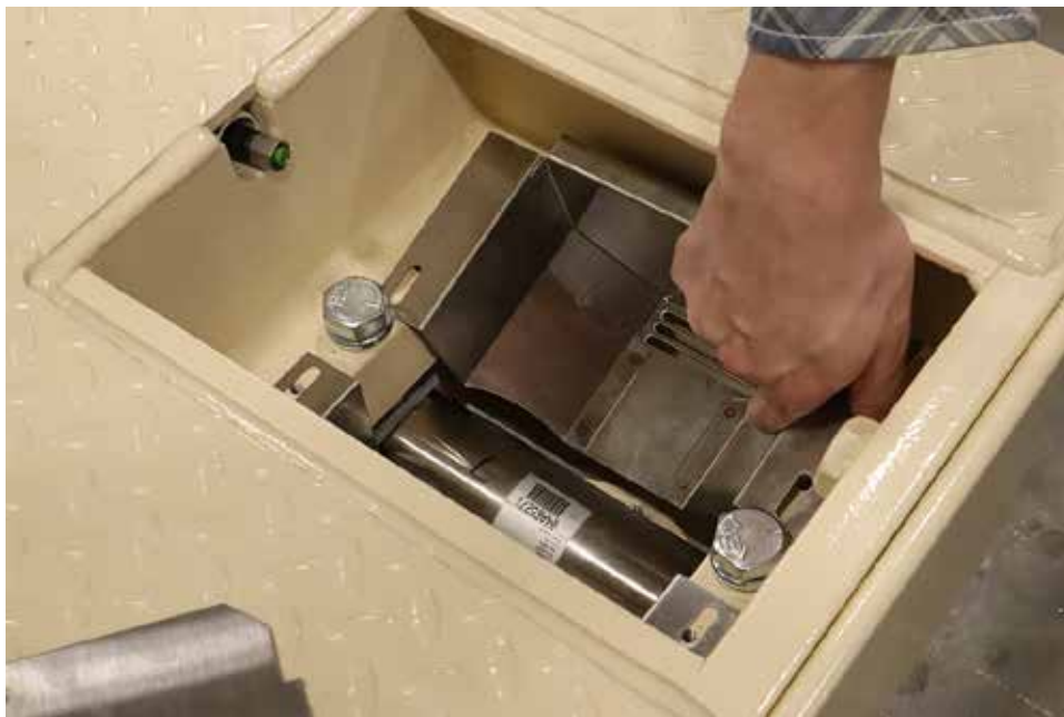
Figure No. 4 – Tilt the second load cell guard at an angle and slide it into the load cell pocket.
