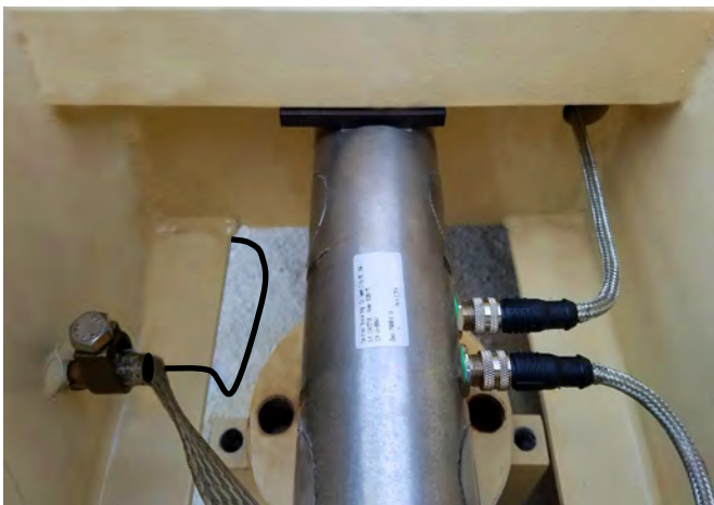
Weighbridge SECTION 2 Ground Stud Connections (Flat Braided Cable and Ground Wire to Indicator)
