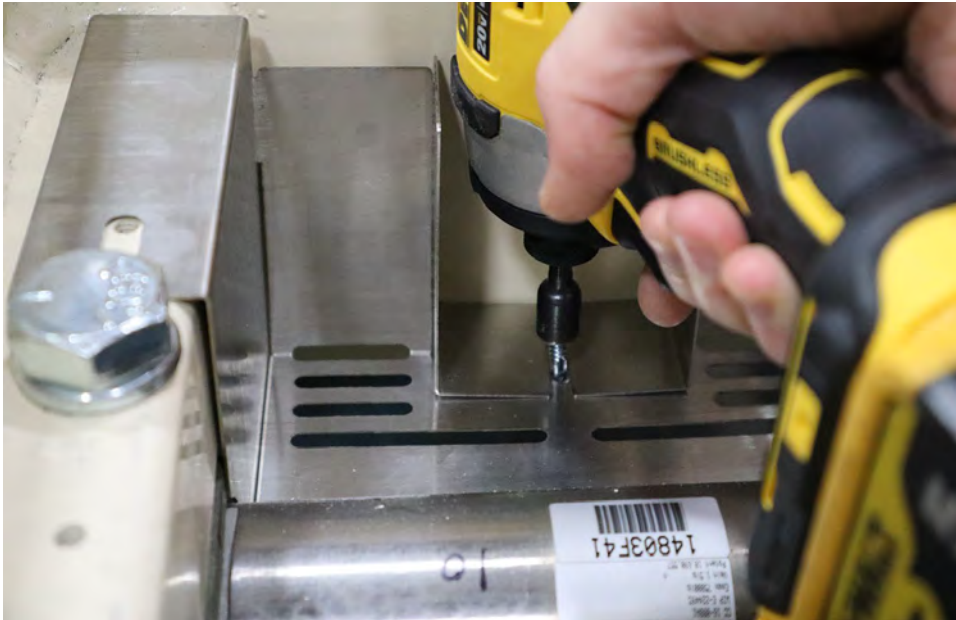
Figure No. 5 – Use the #10 x .75 in self-tapping screw to secure the inner guard plate to the inner load cell guard.
