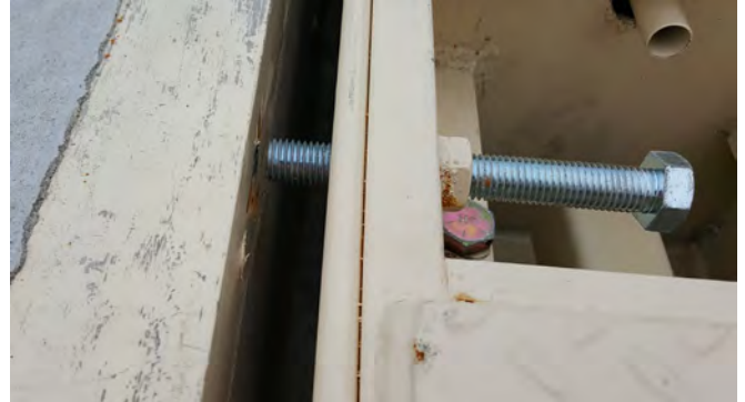
The alignment bolts must be removed before scale calibration and operation.
