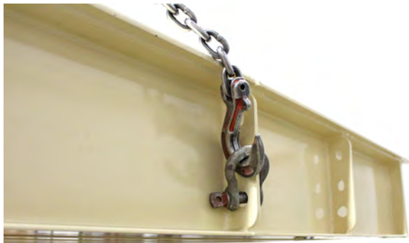
Hook-on and hook-end bridges have an additional guide rail bracket that can be used when lifting by a crane.
