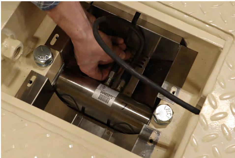
Figure No. 6 – Connect the digital load cell cables to the load cell.
