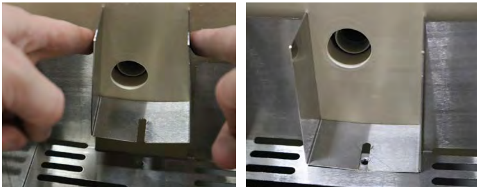
Figure No. 4 – Install the inner guard plate and align the slot with the hole in the inner load cell guard.
