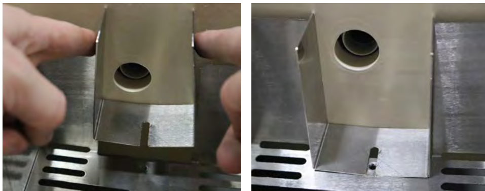
Figure No. 6 – Install the inner guard plate and align the slot with the hole in the inner load cell guard.
