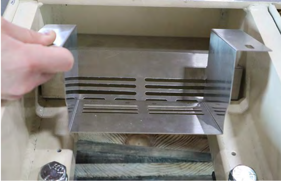
Figure No. 7 – Tilt the outer load cell guard at an angle and lower it into the load cell pocket.
