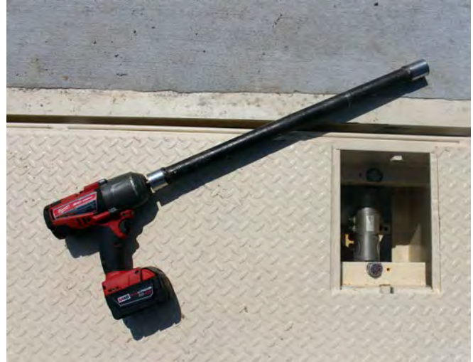
The impact wrench used to install anchor bolts must have a 3000 to 4000 in-lb torque rating.
