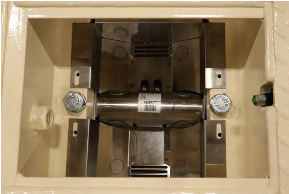
Figure No. 5 – Second load cell guard installed and positioned over threaded holes.
