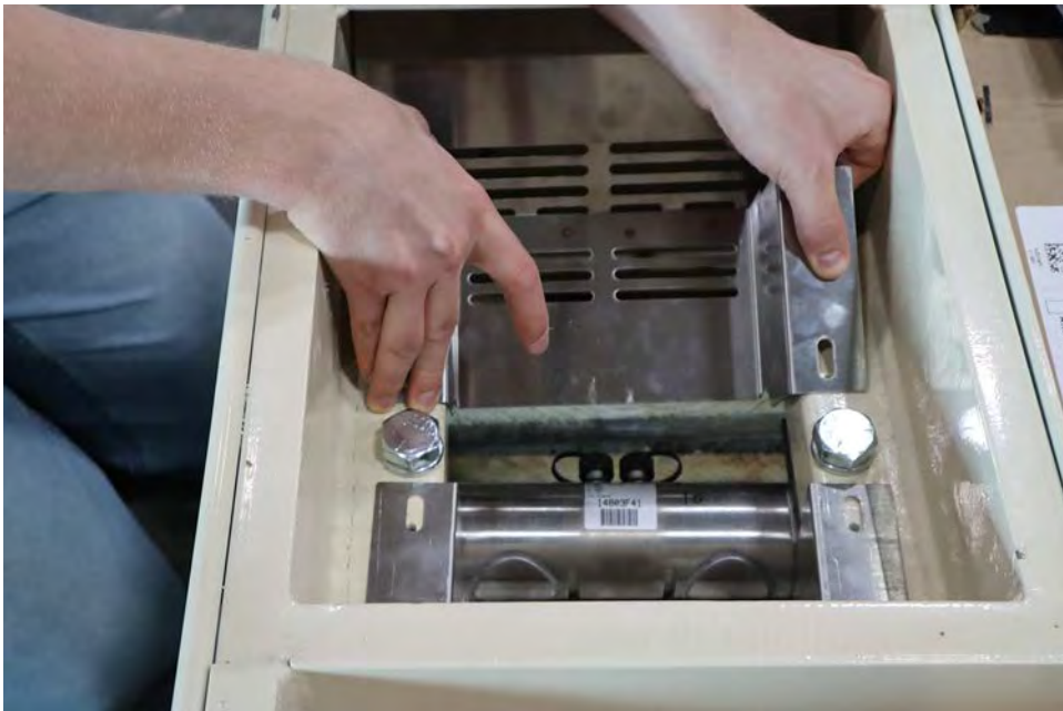
Figure No. 8 – Push the outer load cell guard into the load cell pocket opening, tilt it at an angle, and then pull it forward under the load cell connectors.
