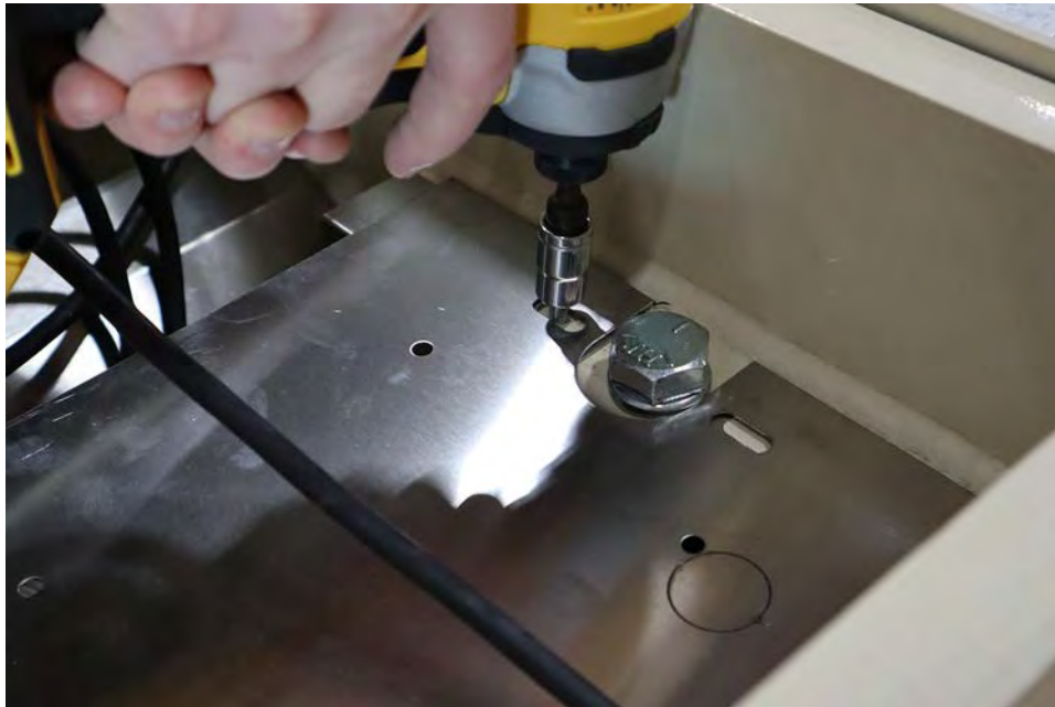
Figure No. 10 – Place the stainless steel cable tray under the cables in the load cell pocket.
