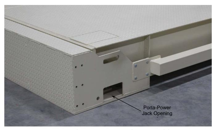
Loosen load cell mounting bolt, and load cell pivot plate retaining bolt, then insert porta-power jack into opening to lift weighbridge to add shims.
