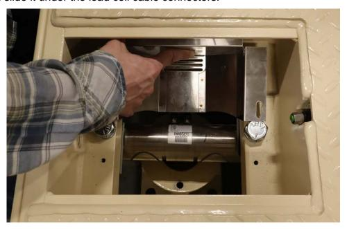
Figure No. 2 – Tilt load cell guard at an angle and slide under load cell cable connectors.
