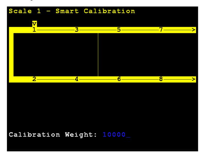
With an empty scale, press **ENTER**. This will capture the calibrated dead load weight of the scale.
