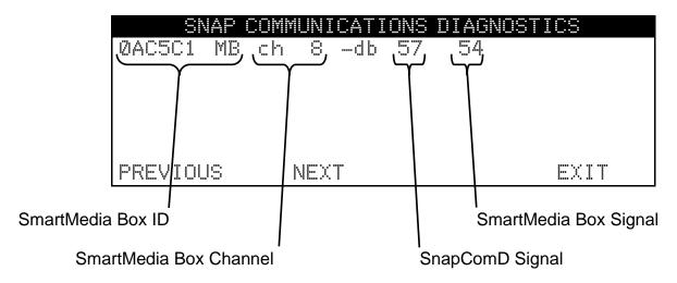
**NOTE:** The –db numbers are the signal strength detected at the SnapComD and SmartMedia Box. Lower numbers indicate better signal strength.
