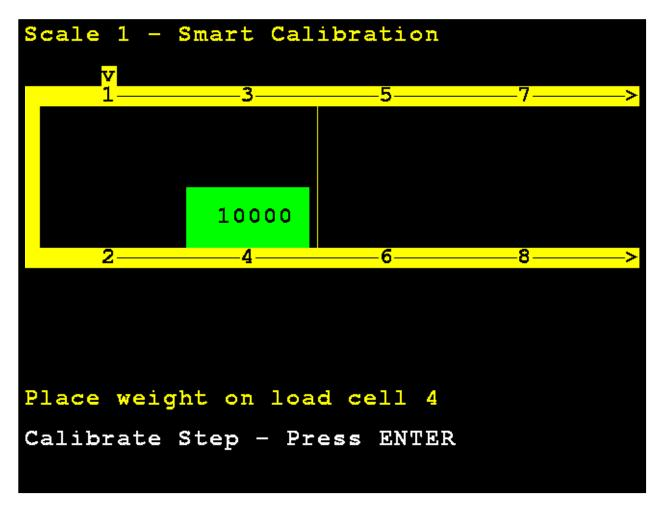
If more than four cells and the number of cells is even a number (such as for an eight-cell scale), the calibration pattern will be the odd number cells, then the even number cells *in reverse* to facilitate easy weight cart movement:
