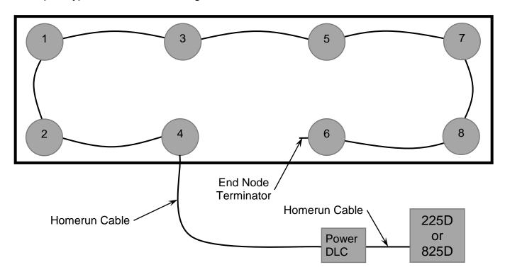
**NOTE:** If the loop were run in the other direction, the sequence would then be 6-8-7-5-3-1-2-4 with load cell 4 having the End Node Terminator installed on it.
