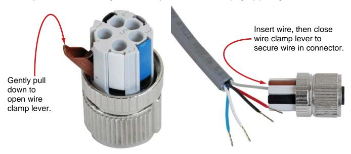
**7.** Repeat steps 4 through 6 until all five wires of the homerun cable are installed in the metal part of the connector.
