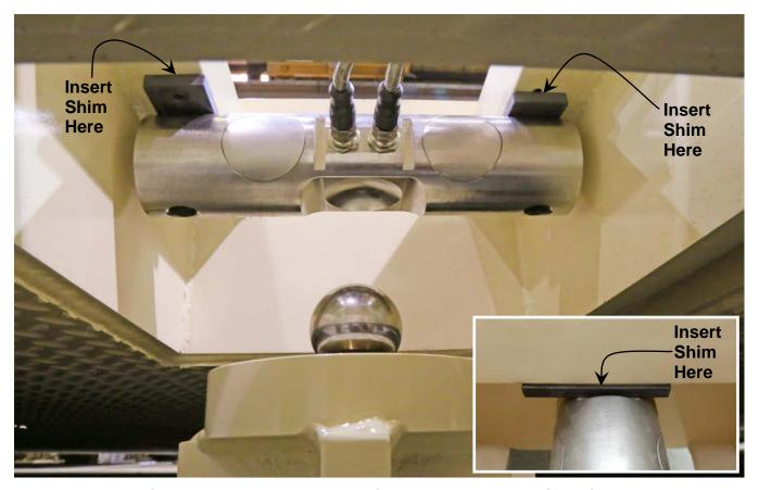
Install shims between the load cell pivot plate and the weighbridge load cell block to evenly distribute the deadload.
