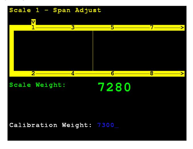
After a brief delay, the span will be adjusted (trim will be adjusted for all cells of the scale) and the 825D display will return to the **Scale 1 - Calibration Options** screen.
