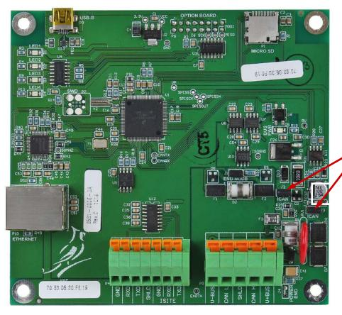
Remove J2, J3 ICAN Jumpers when using POWER-DLC
