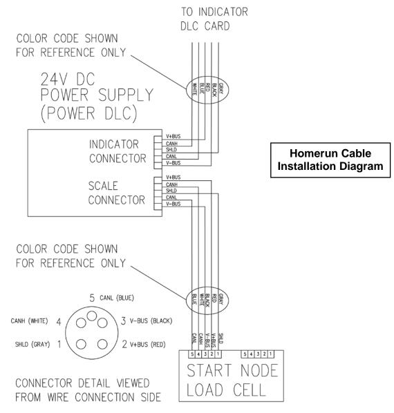
The main (longer) section of the Homerun Cable is connected to the first load cell in the loop (the Start Node) and the SCALE terminal block in POWER-DLC. An additional (shorter) section of Homerun Cable is then connected to the INDICATOR terminal block in the POWER-DLC and the indicator DLC card.
