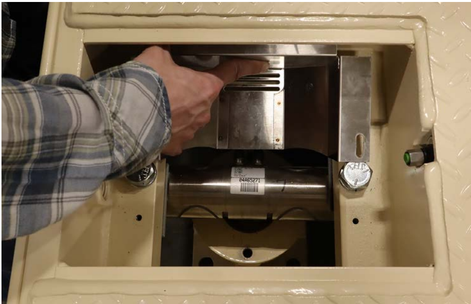
Figure No. 2 – Tilt load cell guard at an angle and slide under load cell cable connectors.
