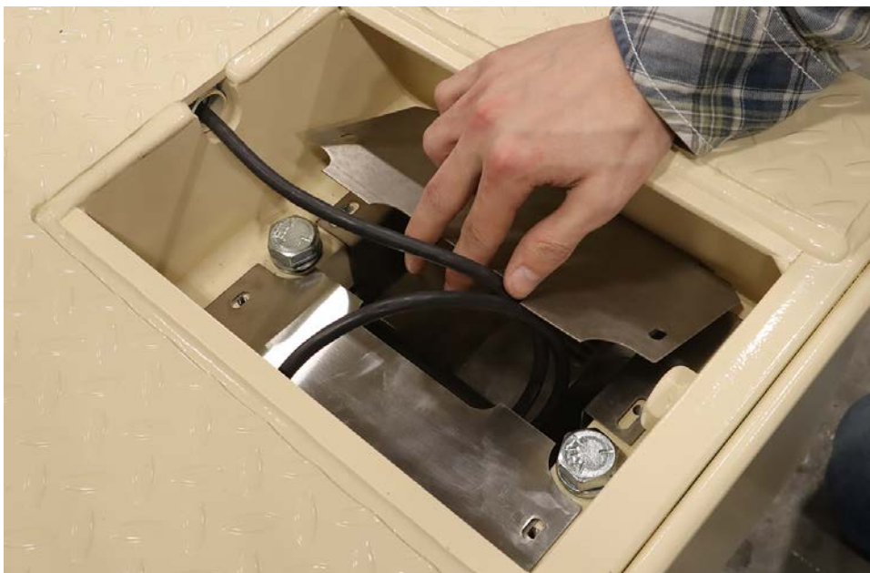
Figure No. 9 – Move cables to the cut-out, then place guard cover into the load cell pocket.
