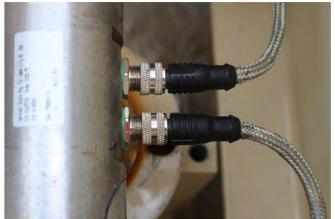
**Install the load cell cable connectors on the load cell fittings and hand-tighten.**
