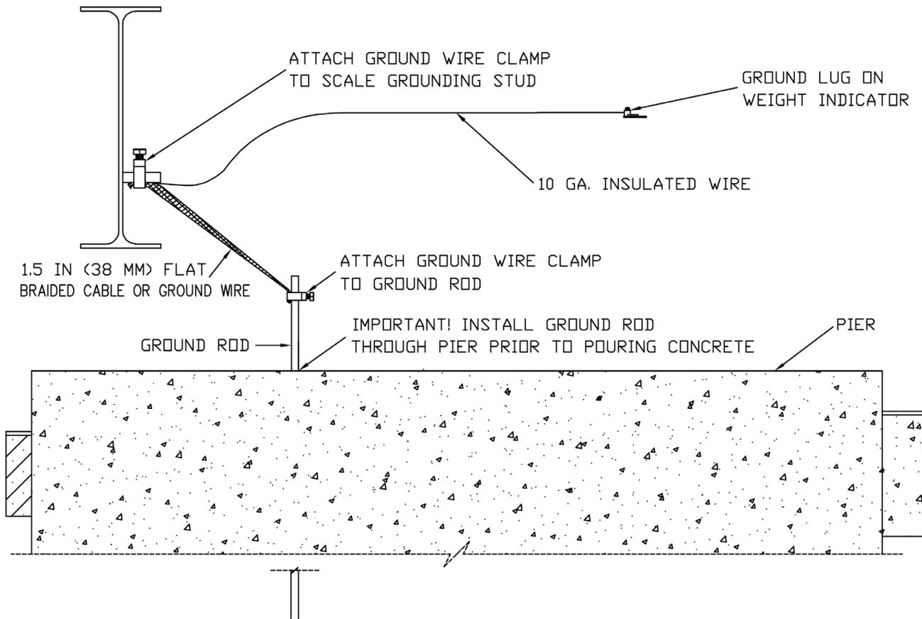
**Diagram of Scale and Indicator Grounding per 3520-0671-GS
