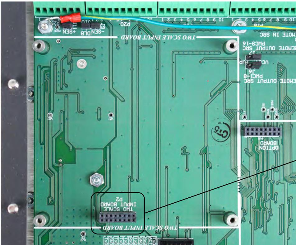
Align pins on 225DLC card with holes in P2.
