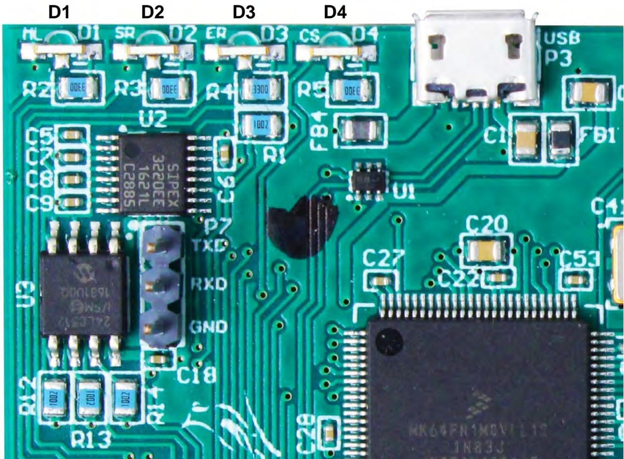
**D1** – Blinking = Indicates the 825-DLC card is communicating with the 825D mainboard.
