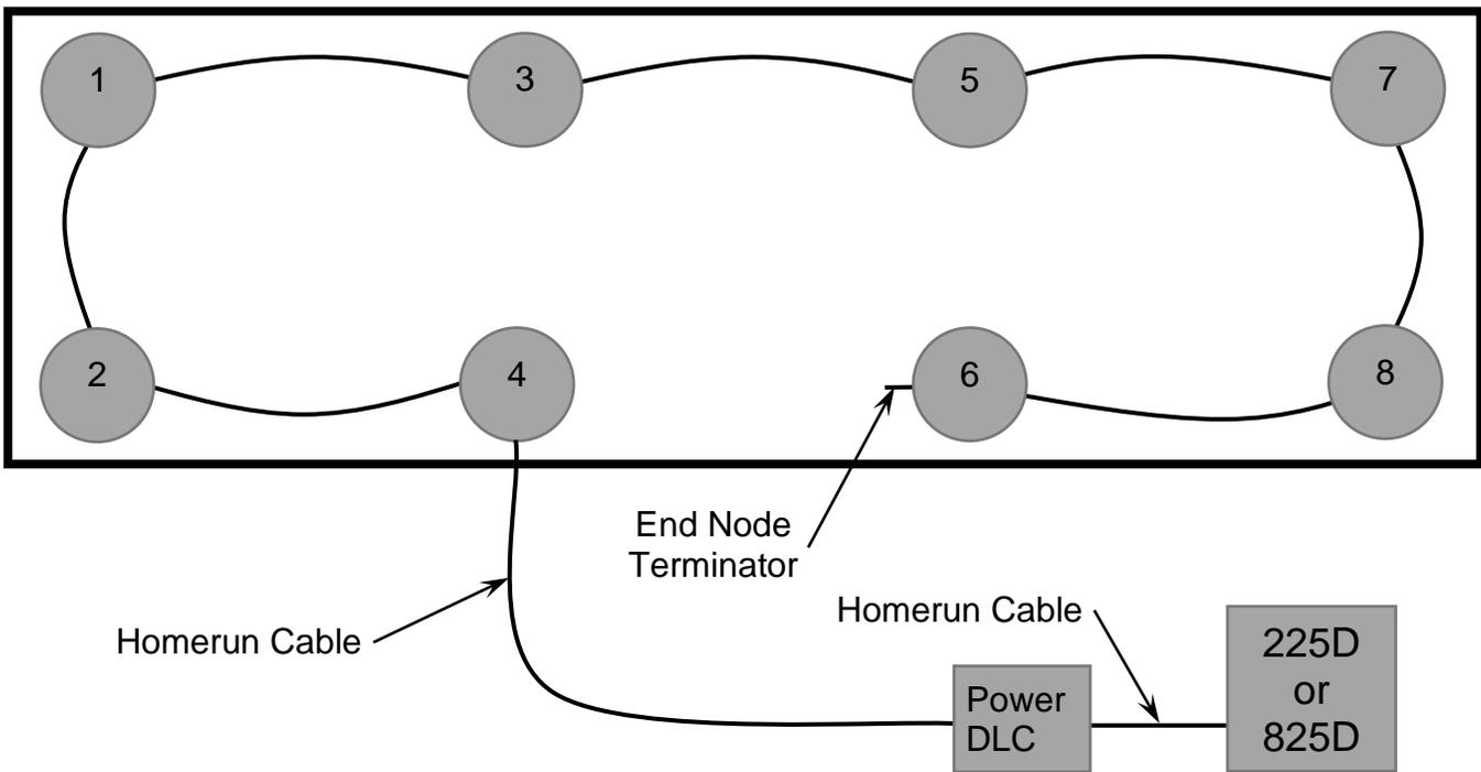
**NOTE:** If the loop were run in the other direction, the sequence would then be 6-8-7-5-3-1-2-4 with load cell 4 having the End Node Terminator installed on it.
