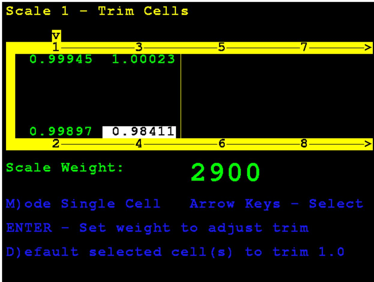
When finished, press, and release the **SHIFT** key, then press the **ESC/←** key to exit.
