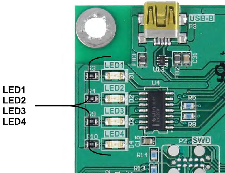
LED1 (RED) – MAIN BOARD TX/RX: Toggles each time the DLC controller and the 225D Mainboard exchange messages.
