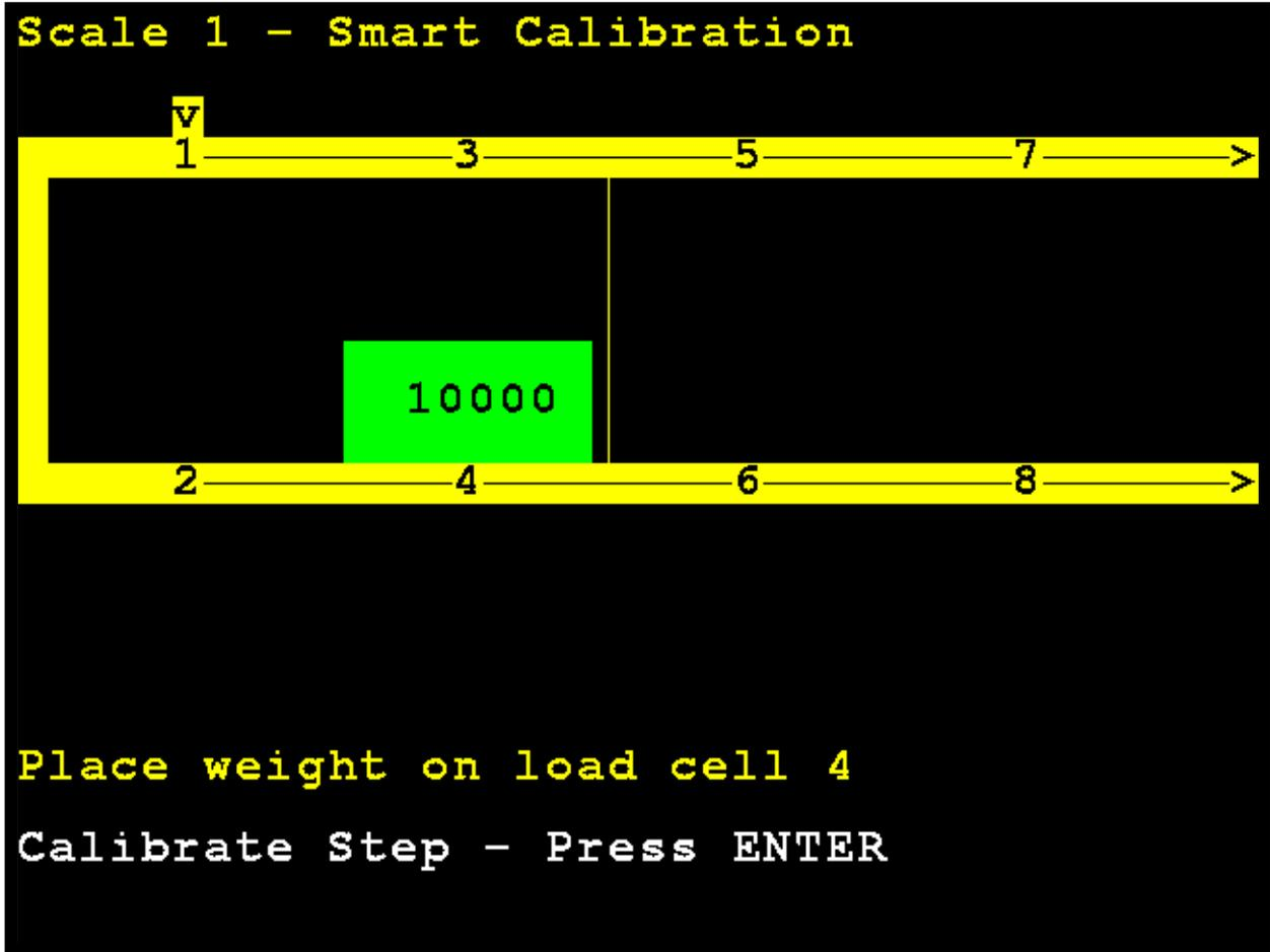
If more than four cells and the number of cells is even a number (such as for an eight-cell scale), the calibration pattern will be the odd-numbered cells, then the even-numbered cells *in reverse* to facilitate easy weight cart movement:
