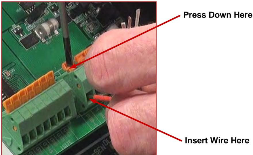
13. Repeat steps 11 and 12 until all five wires of the homerun cable are installed in the P5 terminal block on the 225DLC controller card.
