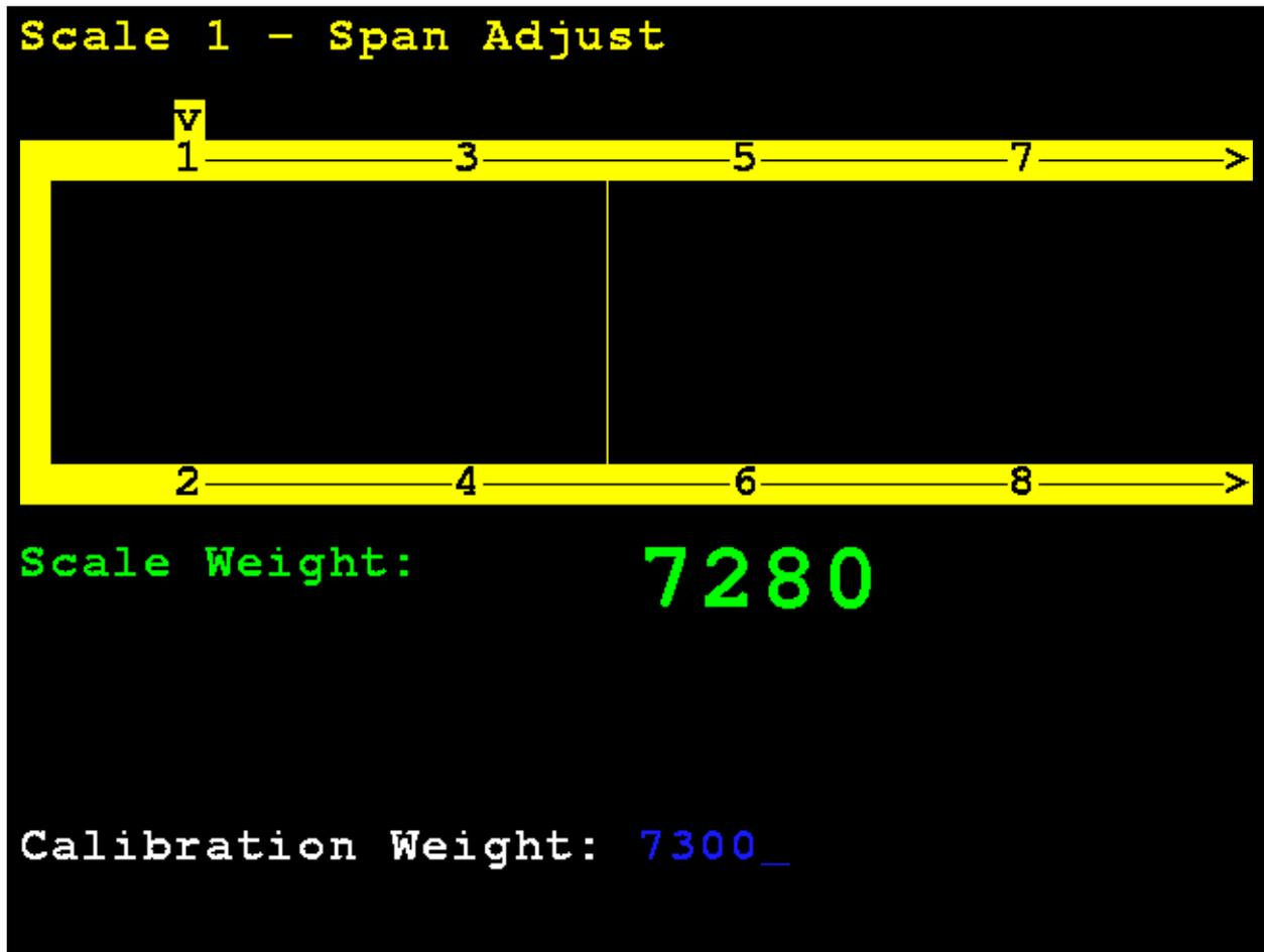
After a brief delay, the span will be adjusted (trim will be adjusted for all cells of the scale) and the 825D display will return to the **Scale 1 - Calibration Options** screen.
