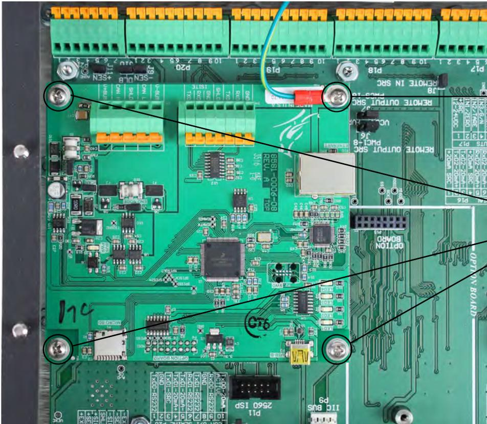
Remove this screw, washer, and the ground wire
