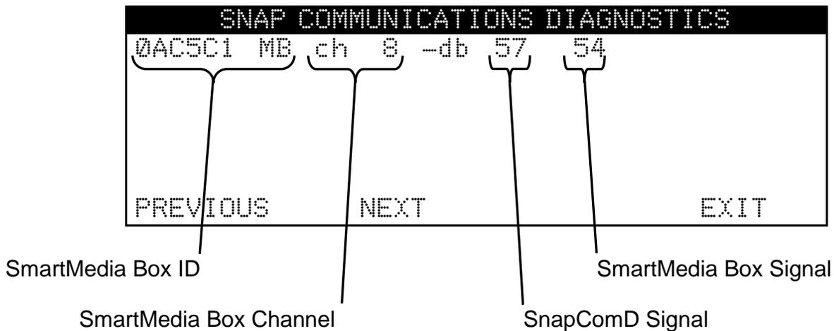
**NOTE:** The -db numbers are the signal strength detected at the SnapComD and SmartMedia Box. Lower numbers indicate better signal strength.
