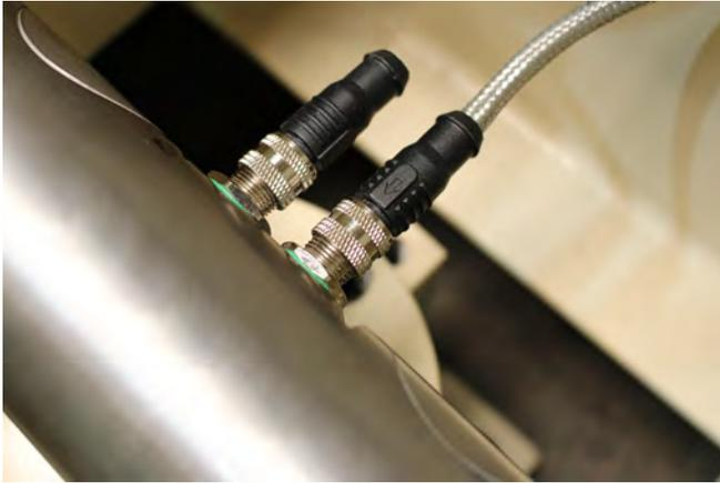
**Install the End Node Terminator on the last load cell of the connection loop.**
