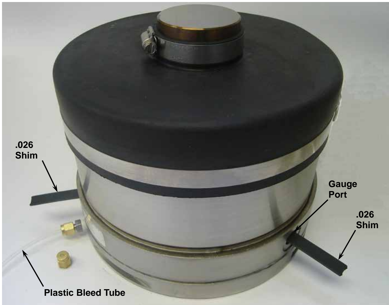
SST75 Hydraulic Load Cell with .026 Shims in Gauge Ports
