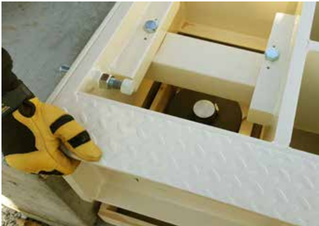
Use a hydraulic jack to lift weighbridge and remove wood blocks, and then lower weighbridge down on the load cell.
