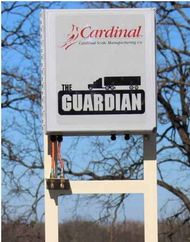
Mount Totalizer Enclosure at least 24 inches off ground to allow room to connect tubing to bulkhead fittings.
