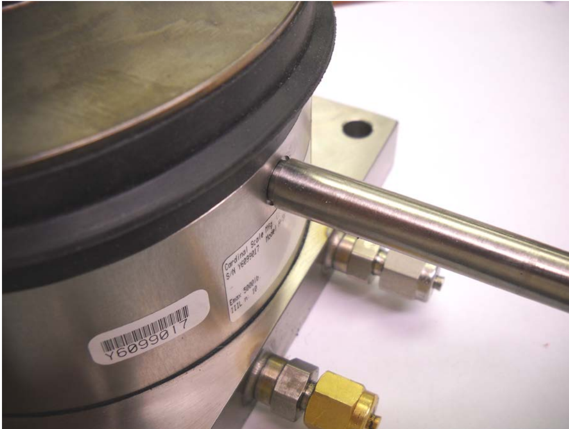
Figure No. 9 (Load Cell with correct amount of oil and Piston at correct height)
