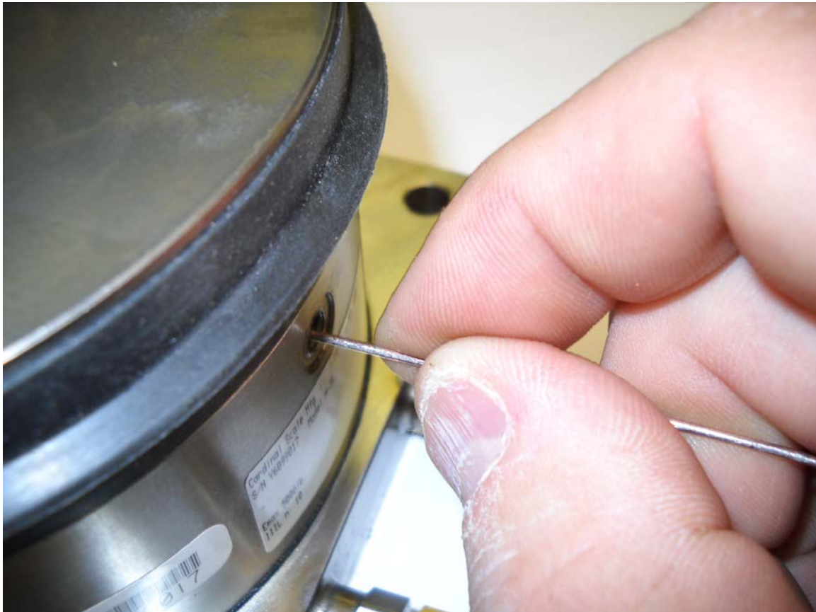
Figure No. 12 – Probing cell gauge port to determine piston position.
