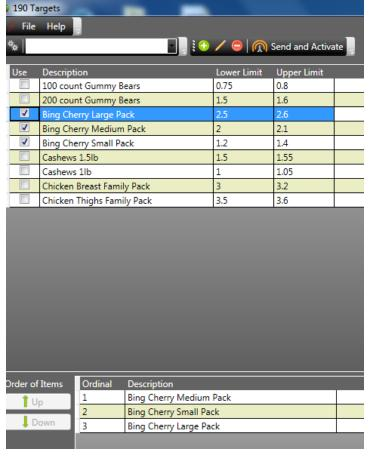
Selecting presets from the database to create a list and then ensuring they are in the proper order before sending it to the 190 indicator.
