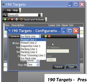
Selecting an indicator (Device) to configure the communication connection from the PC to the 190.
