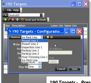
Selecting an indicator (Device) to configure the communication connection from the PC to the 190.
