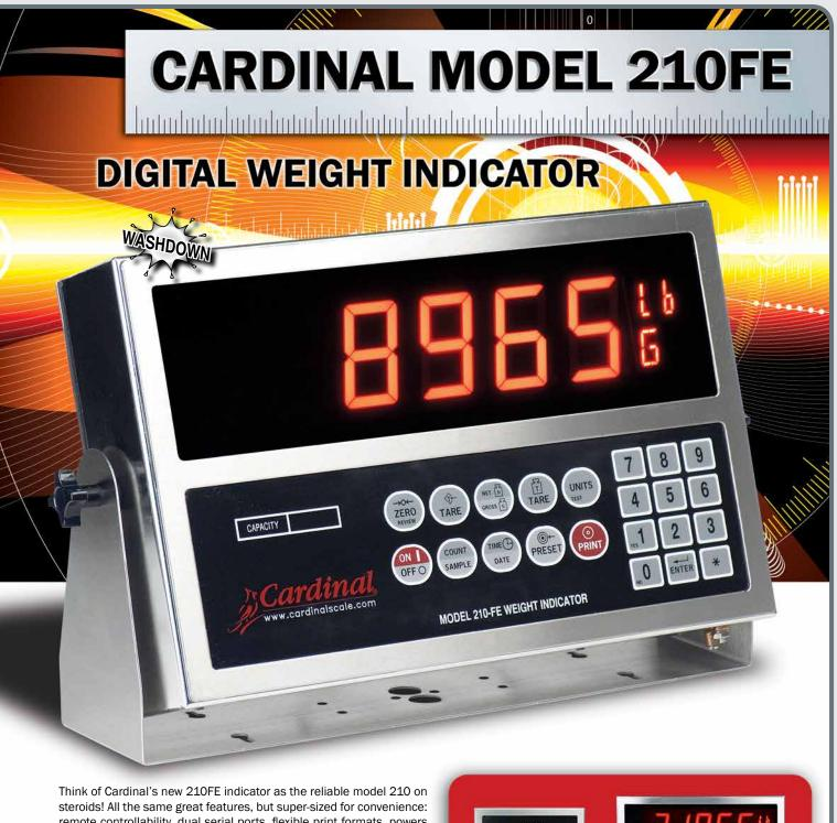
steroids! All the same great features, but super-sized for convenience: remote controllability, dual serial ports, flexible print formats, powers 8 load cells, numeric keypad, auto shutoff, and selectable key lockout all in a 15-inch-wide by 9.7-inch-high stainless steel enclosure with 2.24-inch-high LED digits and larger key sizes.
