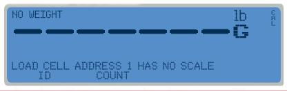
**PROBABLE CAUSE:** A load cell has not been assigned to a scale.
