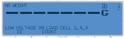
**PROBABLE CAUSE:** Low power on a load cell. Load cells at the end of the CAN daisy-chain are most susceptible to low voltage errors because of voltage drop along the cable.
