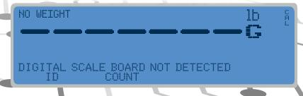
**PROBABLE CAUSE:** The indicator cannot communicate with the option card or the option card is not responding.
