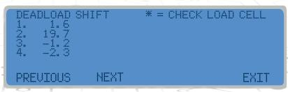
This shows the live shift from the original calibrated deadload. An asterisk (\*) indicates that the deadload shift has been exceeded. Scale must empty for this to be valid.
