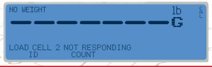
**PROBABLE CAUSE:** The indicator cannot detect the exact communication problem with the unresponsive load cell.
