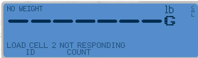
**PROBABLE CAUSE:** The indicator cannot detect the exact communication problem with the unresponsive load cell.
