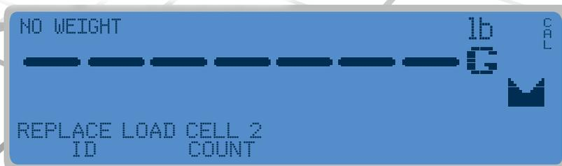
**PROBABLE CAUSE:** There is irreparable internal damage to the load cell.
