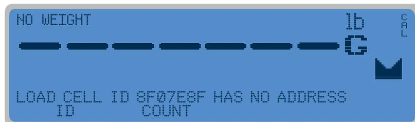
**PROBABLE CAUSE:** A load cell is responding but it is not addressed in the system.
