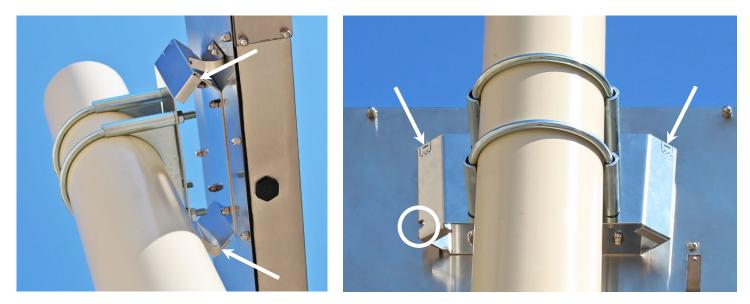
5. To secure the SB600 in the pole bracket, there are tabs on each end of the bracket that can be bent over to secure the SB600 in place. Simply insert a flat-blade screwdriver in the slot and lift up and forward towards the SB600. To further secure the SB600 in the pole bracket (*and to prevent theft*) both brackets have a security hole in which a padlock can be installed.
