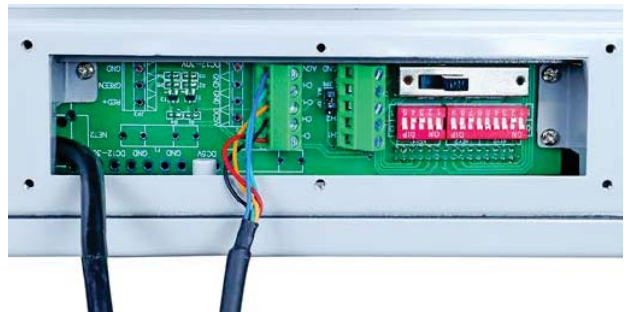
Figure No. 5 Lower the Access Panel to allow access to the configuration switches.
