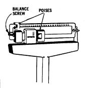
To balance scale move both poises to zero (0) and turn bal-
