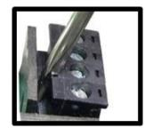
Remove the connector using a small flat-blade screwdriver as shown to avoid pin damage. (B) IF 10-30 VDC power Supply is connected Remove the DC supply Power Connector inside the Integrator.
