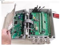
Remove the 4 screws in the mounting plate Leave the Terminal and Sensor Board attached to the mounting plate
