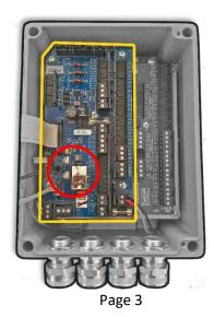
3. Make sure the fuse fits snuggly in the fuse clip! If the fuse is loose, remove it and compress the fuse clip contacts to make a tighter fit.
