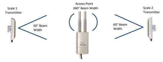
Transmitters installed at different elevations.Angle directional antennas to focus the signal at the omnidirectional antennas.
