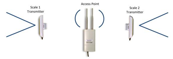
2. Poor line of sight causes low signal strength and connection failure.
