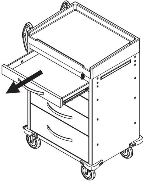
② Push release levers in middle of both slides, one up and one down.
