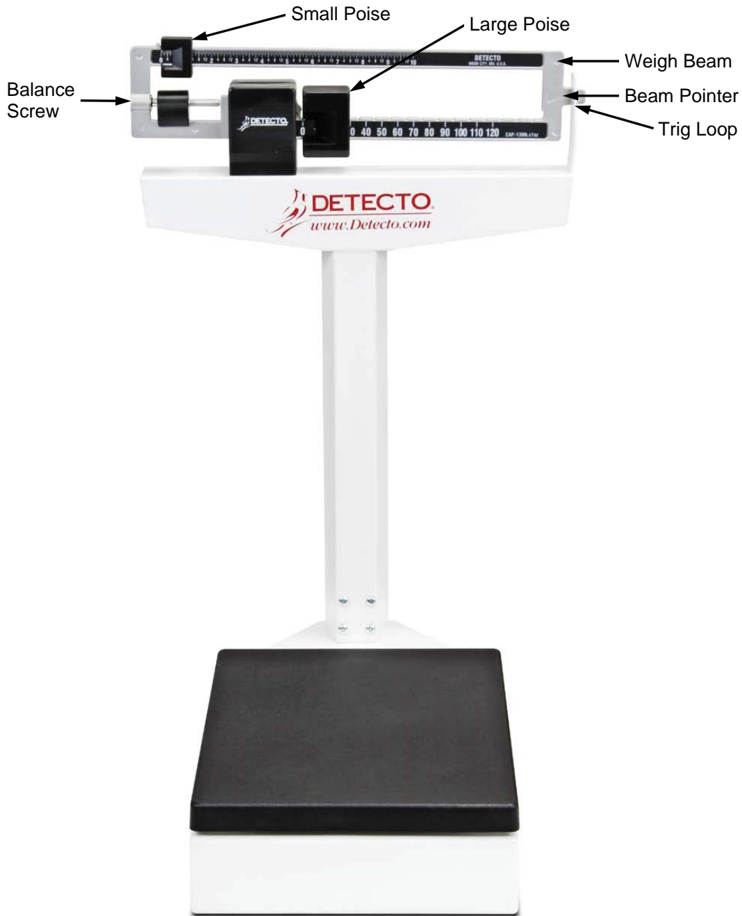
Figure 7 - View showing components for balancing scale prior to normal operation.
