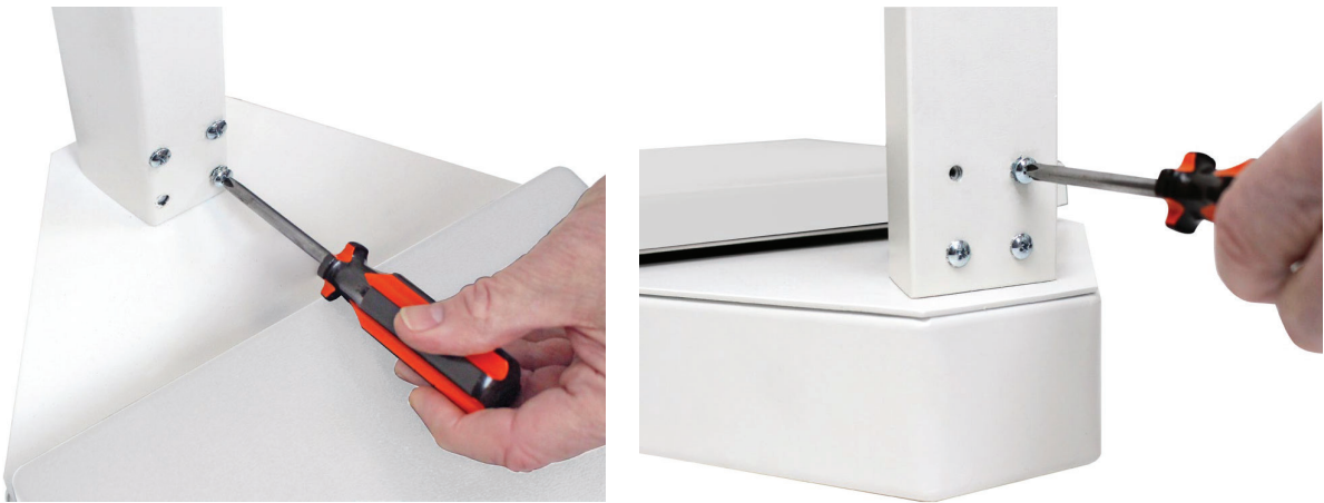
Figure 2. - Install eight screws and washers to secure column to scale base
