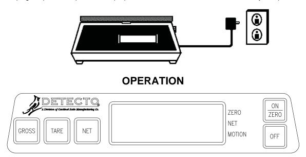
When applying power, make certain the scale platform is empty. Press and hold the **ON/ZERO** key until one of the annunciators (ZERO, NET or MOTION) turn on. When one of the annunciators turn on, release the **ON/ZERO** key. After a second or so the display should indicate a zero weight with the ZERO annunciator turned on. Weighing may now begin. If the display does not indicate zero, press the **ON/ZERO** key again to zero the weight display.
