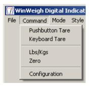
◆Push-Button Tare - This command performs the same function as the PB Tare button on the keypad.
