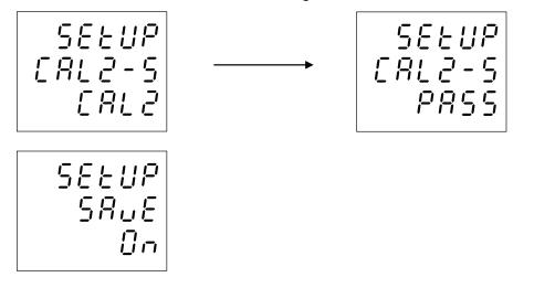
Remove the calibration weight from the remote scale platform
