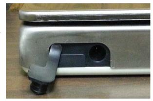
5 hours to fully recharge the battery pack in the scale. While the batteries are charging the WPS12 can still be operated.
