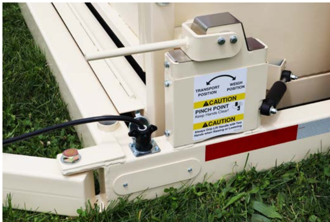
Front Cam lever in Transport position.
