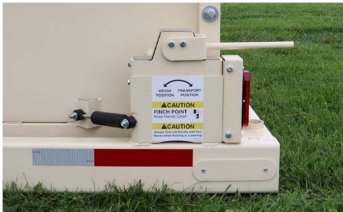
Rear Cam lever in Transport position.
