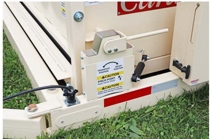
Front Cam lever in Weigh position.
