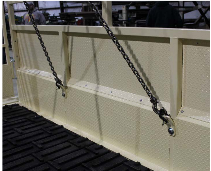
Lifting lugs are spaced to allow balanced lifting of scale.
