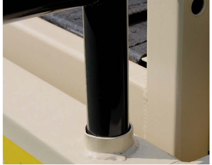
Insert Gathering Panel tube into frame opening.
