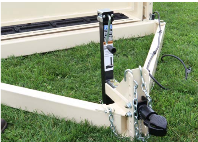
Lower scale tongue arms until they are on the ground using the scale hitch jack.
