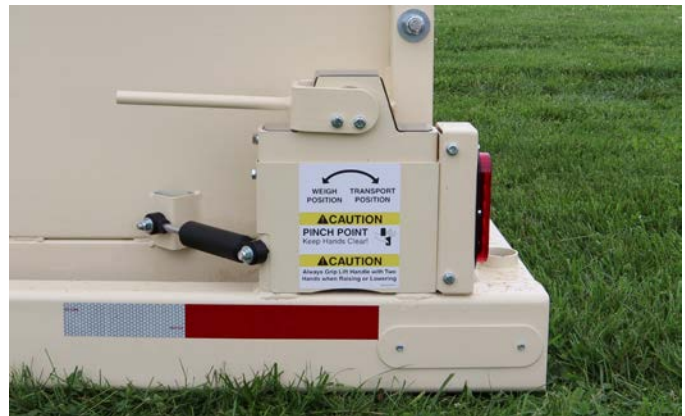
Rear Cam lever in Weigh position.
