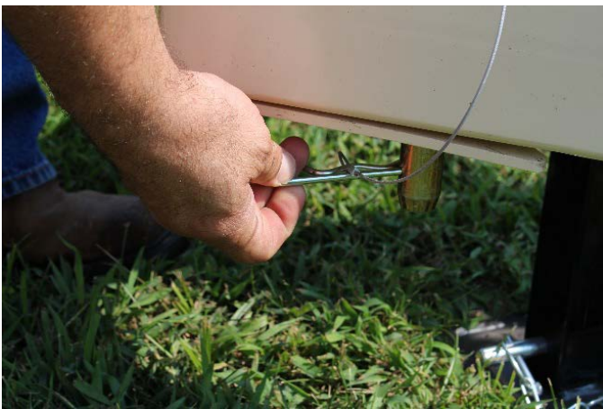
Remove retaining clip securing safety pin.
