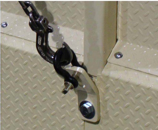
Only lift the scale with the installed lugs.
