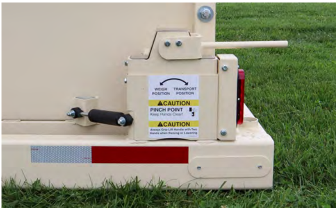
Rear Cam lever in Transport position.
