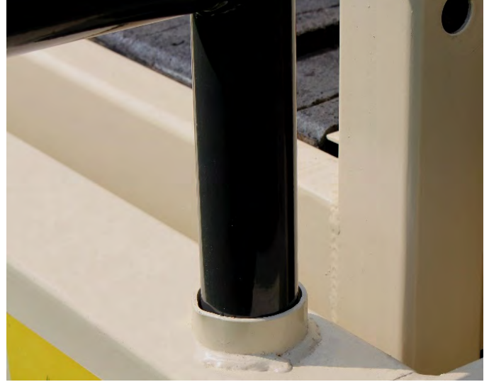
Insert Gathering Panel tube into frame opening.
