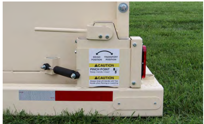
Rear Cam lever in Weigh position.
