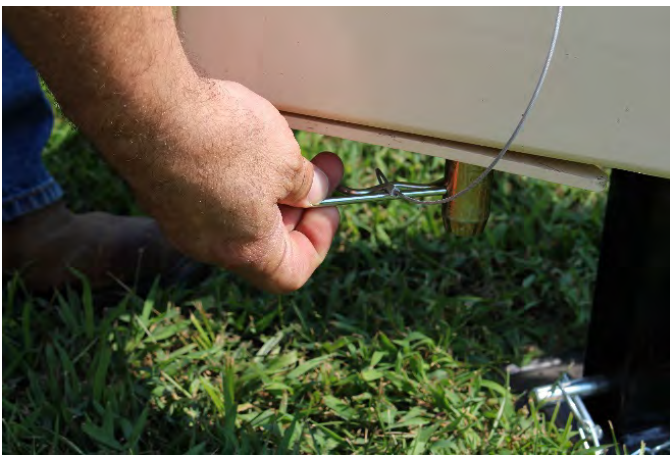
Remove retaining clip securing safety pin.
