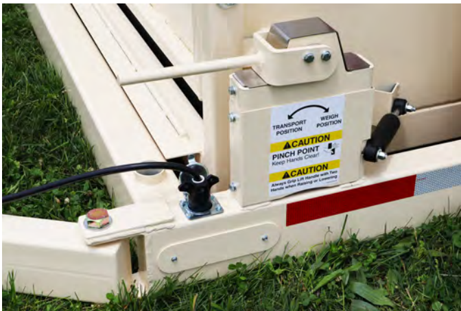
Front Cam lever in Transport position.
