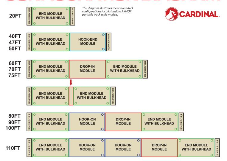
The drop-in module for the deck acts more or less as a bridge in the middle of the deck without load cells, and the drop-in module length can be varied to reconfigure the scale bulkhead modules to fit a weighing requirement. Drop-in modules have been historically 20ft in
