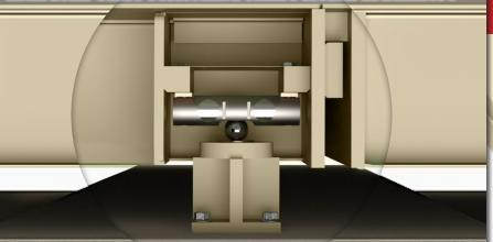
There are no moving parts below the ARMOR® weighbridge, including the load cells, which eliminates build-up failures due to corrosion, sediment, and debris. The axis® load cell stands are fabricated from one-inch-thick steel to minimize rust and corrosion damage and ensure long-term strength and durability.
