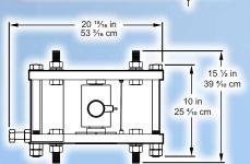
These sizes shown in the diagram are for 50K, 100K, and 120K SCA load cells. Consult factory for 200K SCA load cell stand dimensions.
