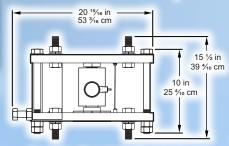
These sizes shown in the diagram are for 50K, 100K, and 120K SCA load cells. Consult factory for 200K SCA load cell stand dimensions.
