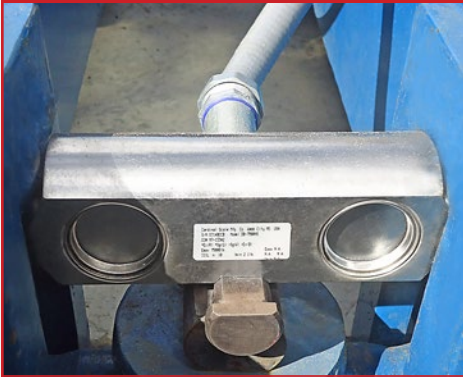
Cardinal Scale's Stainless Steel, Double-Ended Shear Beam, High-Capacity Load Cell
