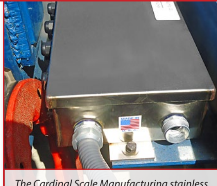
The Cardinal Scale Manufacturing stainless steel junction box provides considerable protection to the electronic components.
