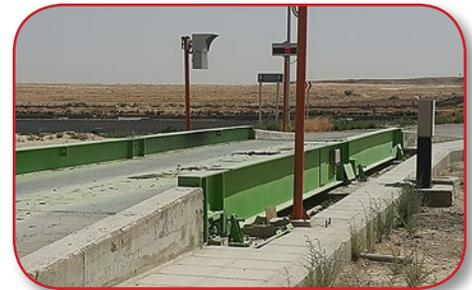
*“Cardinal Scale’s authorized dealer, Traffic Tech, assisted with the project using Cardinal Scale’s load cells, two SB500 remote displays, an unattended 825 indicator in conjunction with Traffic Tech’s weighbridge, camera system, printer, and RFID for driver identification.”*
