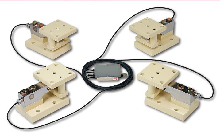
Cardinal Scale's THBC electronic tank weighing systems provide 4 mild steel stands, each with stainless steel, model SB 20,000-lb-capacity load cells wired to a central stainless steel junction box. This 80,000-lb capacity load cell kit features a rugged bolt-in design and self-checking stands with waterproof load cells. The entire system is manufactured at Cardinal Scale's factory in Webb City, MO.
