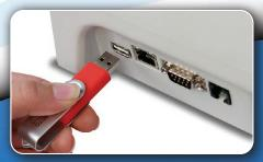
The DL series scales' USB drive allows you to download PLUs, shortcut keys, and other setup information, including custom labels, to the scale. Upload these same items from the scale to the USB drive which can be viewed in the included utility software.
