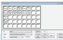
This graphic display allows PLUs to be quickly assigned to quick keys. This page can then be printed and used as the quick key overlay for the DL Series scale.
