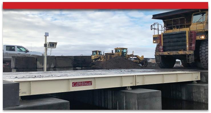
The specs on this installation are enough to make any heavy-capacity scale aficionado salivate: twin digital YUKON off-road truck scales (for haul trucks weighing up to 300 tons) and a Satellite 825D indicator connected to a long-range RFID tag reader for completely-unattended data transactions. The system consists of two checkered steel deck 30 ft x 12 ft YUKON
