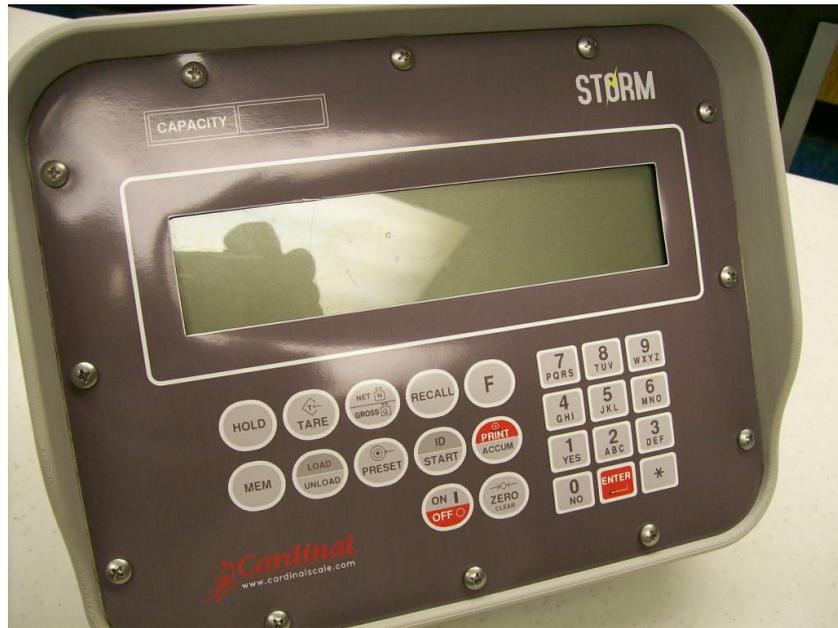
**Figure 7** Model 212G Front panel
