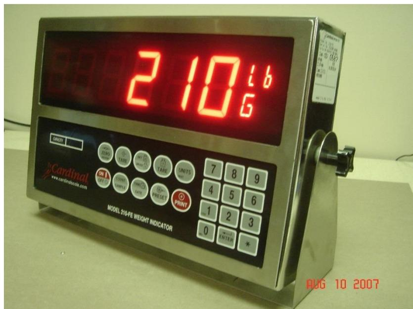
**Figure 5** Model 210-FE Front panel
