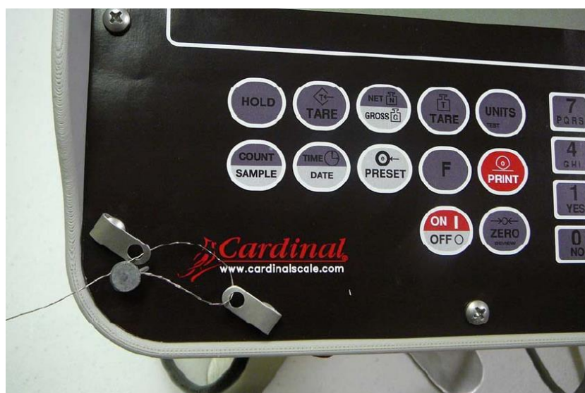
Figure 10 Sealing of Model 212G / 212GX with wire and seal.
