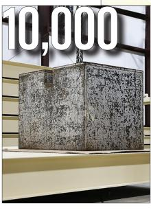
A massive 10,000-lb test weight is applied to each ARMOR® SmartCell® load cell in its respective quadrant. This test weight is meant to emulate a real-world weighment and prepare the scale for practical accuracy. Every ARMOR® digital truck scale is 100% factory calibrated and tested prior to shipment.
