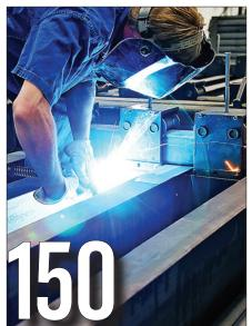
Cardinal Scale's experienced welding team applies 150 tack welds to hold a 70-foot ARMOR® truck scale weighbridge in place. This large number of carefully-placed welds guarantees final welds that are applied will be completed perfectly.
