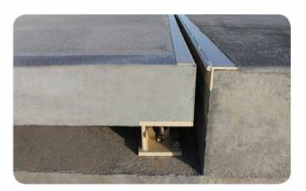
The Harvester® truck scale's factory-poured precast concrete decks are 7.25 inches thick for optimum strength, and the entire scale is only 14.75 inches high from the top of the pier to the top of the scale deck for a low profile.
