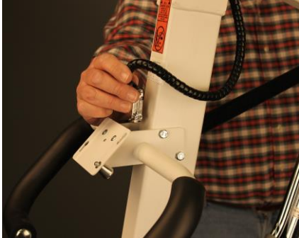
Route cable around boom...
