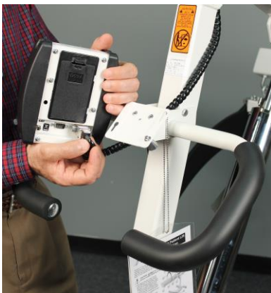
Install load cell cable and secure with cable connector retaining screws
