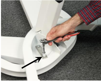
Remove mounting bolt
