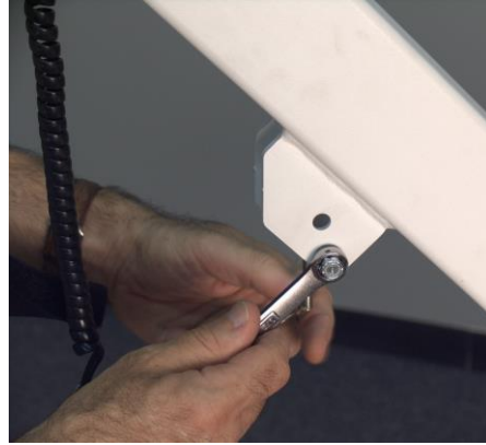
Remove Bolt, Washer & Nut
