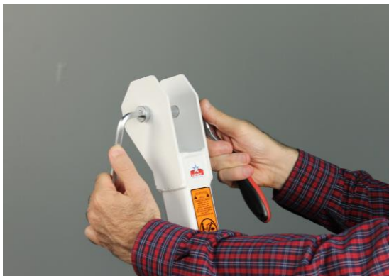
Remove Bolt from Column
