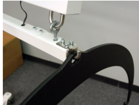
Completely tighten all three retainer plate screws
