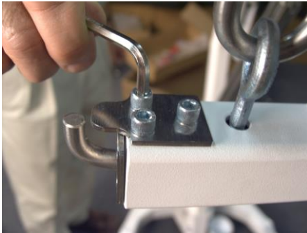
Remove outer 2 Screws Loosen inner Screw
