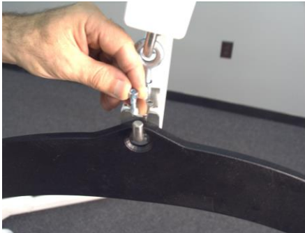
Lift hoop slightly to ease screw installation
