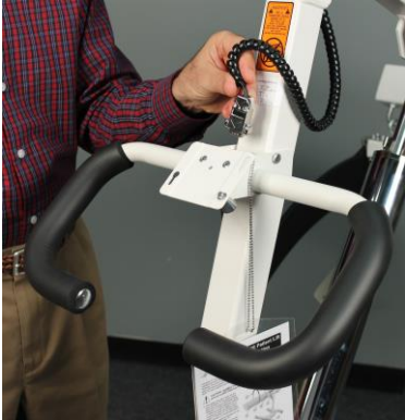
Route cable around boom...
