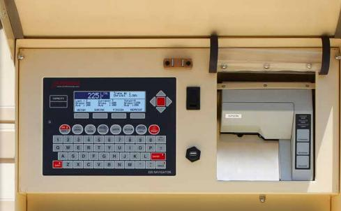
Cardinal Scale's legal-for-trade 225 digital weight indicator, USB drive port, and CTP-1 ticket printer combine in the weatherproof, outdoor enclosure of the Weight Wrangler's mobile weighing center.
